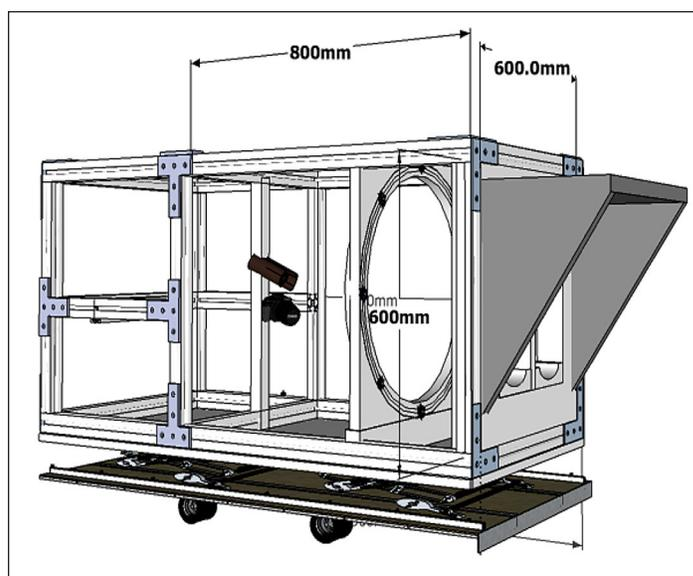
**Figure 1.** Schematic drawing of the interior of the experimental setup. The feet are positioned on the support bars, below the light shield, on the right side of the image. The thermal camera and the color image camera are placed 800 mm from the foot supports, with the thermal camera above the color image camera. The light module is the ring between the cameras and the foot supports, containing eight light-emitting diodes (black dots).
